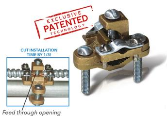
Westgate's new feed-through armored ground clamp saves time, labor and material by allowing you to feed armored ground through the clamp and onto the next connection. Ground wire does not get cut! Cut only the outer armored jacket and insert ground wire into center lug. Secure each side of the armored jacket into the strain reliefs located on each side of the clamp.
