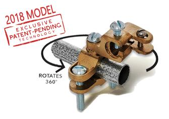
Westgate upgraded MVP98 model "MVP99-360-1C" offers 360 degree rotatability with 1 armor clamp to be installed at the end of the run so armored ground cable could be fed from any direction, reducing cable run, simplifying installation and saving time. The upgraded model also makes tightening of the armored cable quick and easy.
