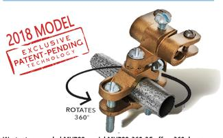
Westgate upgraded MVP99 model MVP99-360-2C offers 360 degrees rotatability with 2 armor clamps to be used in the middle of the run so armored ground cable could be fed from any direction, reducing cable run, simplifying installation and saving time. The upgraded model also makes tightening of the armored cable quick and easy.
